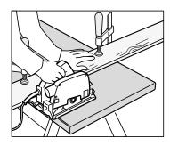
Use a circular saw and G clamps to hold a straight-edge to your pre-cut worktop when you cut to customising the size. It's helpful to use a pair of sawhorses to help you. A tip is to have a second person holding the piece to be cut off to avoid the edge from splintering.
