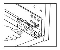
Fasten your drawer slides, starting with your outer drawers. Outer drawer slides should be attached to the outer row of holes in your cabinet.
