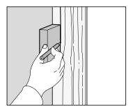
If the wall isn't level and flat, the filler piece must be cut to fit to the wall's shape. To do this, you'll need a filler piece, measuring tape, small block of wood about 2.5–3.5 cm thick and pencil.
