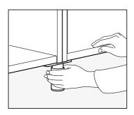
Check that each cabinet is aligned with the previous cabinet by adjusting the legs.
