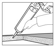
To prevent moisture from penetrating the worktop apply polyurethane silicone across the sawn edges.
