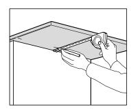
Proof measure your worktop. if you have a pre-cut worktop now is the time to cut it to the right length. To avoid splinter, cut with the worktop underside facing up when using a buzz or jig saw, but with the top if using a handsaw.
