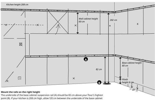
suspension rail and the underside of the rail for the wall/high cabinet. (If the kitchen is 228 cm or 248 cm high you should allow 140 cm or 160 cm respectively.)
