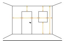
**04** Measure each wall fully from floor to ceiling and from doors to windows. Remember to include door and window frames.
