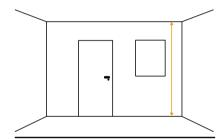
**03** Measure the floor to ceiling, marking the highest and lowest points.
