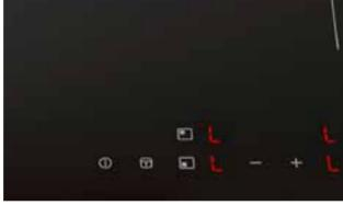
When you press and hold the **child lock** button, you can't start the hob or change the temperature. To unlock the hob, press the child lock button again for 4 seconds. This is also a good function to use when you're cleaning the hob surface and don't want to switch on any zones.
